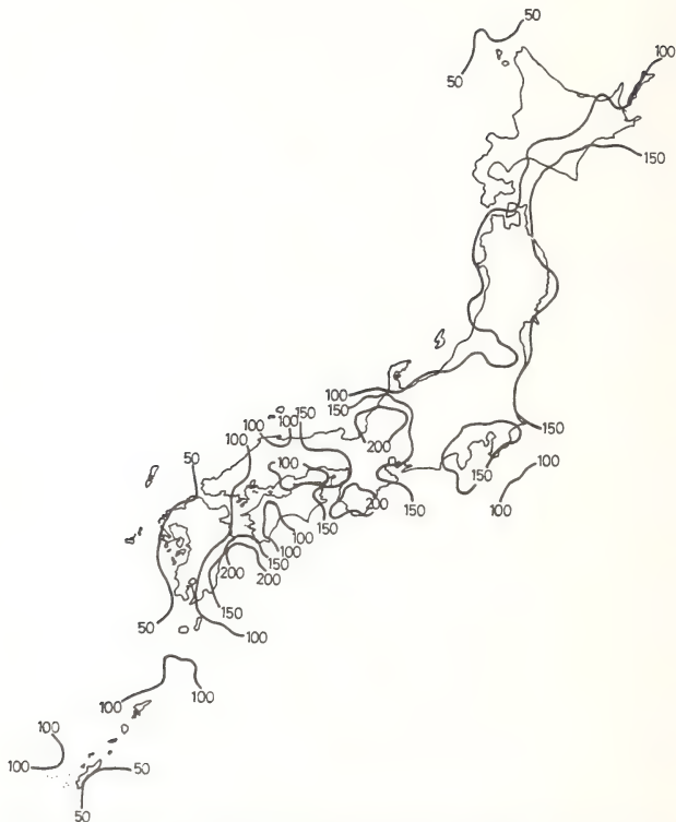
Fig. 8. Regional Distribution of the Expected Maximum Acceleration Values (gal) at the Free Surface of Ground ( T_G=0.3 sec., \tau=50 years)
